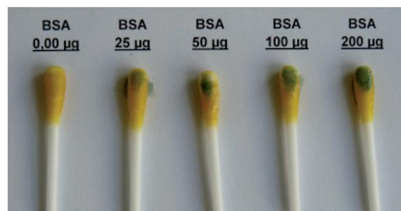
Fig. 3: Colorimetric reaction of RIDA<sup>®</sup>CHECK indicator swabs after wiping the sampling areas which had been contaminated with the protein standard solutions
