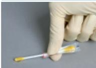
Firmly wipe the surface with the unpackaged part of the RIDA<sup>®</sup>CHECK indicator (Test 1)
