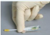
Remove the packaging of the second indicator and firmly wipe the surface of another sampling area (Test 2)
