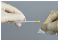
Hold the swab on one side with one hand and remove the other side of the packaging with the other hand
